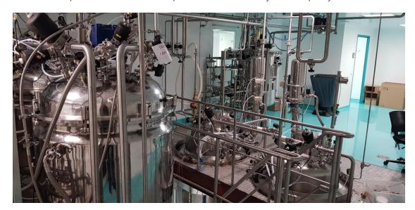
In addition to the bioreactors, manufacturing line also includes a CIP/SIP system.
