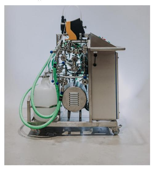
This CIP (Cleaning-in-Place) system is designed to be mobile and can be easily moved between production units. It can be connected to fermenters or other technological vessels and can achieve a maximum detergent circulation speed of 5000 L/h, ensuring fast and efficient cleaning.
