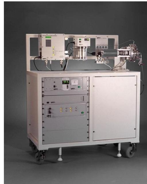
For flow rates up to 12 l/min, the QIC MultiStream can measure selected stream flow rate.
