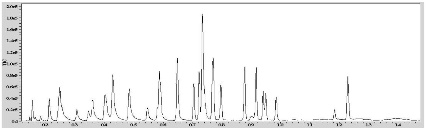
**Figure 1** – Total ion chromatogram of a 100 ppb sample of the calibration mix as given in Table 1
