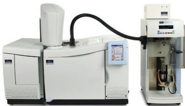
Figure 1. Clarus 600 GC/MS interfaced to the Pyris 1 TGA.
